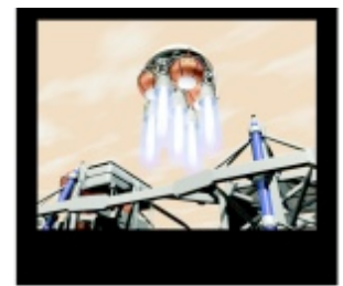
The CLV & ISPP provides LOX/CH 4 propellant to the ascent Crew Vehicle. The ascent Crew Vehicle will rendezvous with the Earth Return Vehicle in orbit around Mars.
